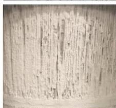
This photo shows a plugged filter cartridge. It can be caused by wet air or simply not operating the vibrator cleaning cycle properly or enough time for 8 hour days.
